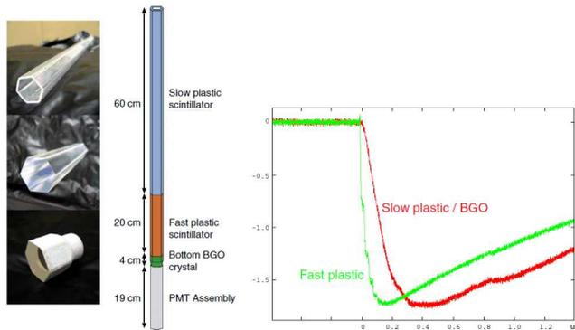
Figure 2. (Left) Structure of the PDC. Fast, slow and BGO scintillators are viewed by one PMT. (Right) An example of waveforms of the PoGOLite CSA output. The decay time of the fast scintillator ( $\tau \sim 2$  ns) is distinguishable from that of the slow scintillator/BGO ( $\tau \sim 300$  ns) (Pulse- Shape Discrimination).
