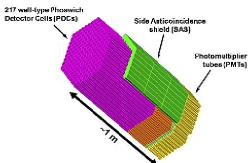
Figure 1. Schematic view of the PoGOLite detector array, consisting of 217 PDCs and 54 SAS units, giving 271 PMT output signals in total.
