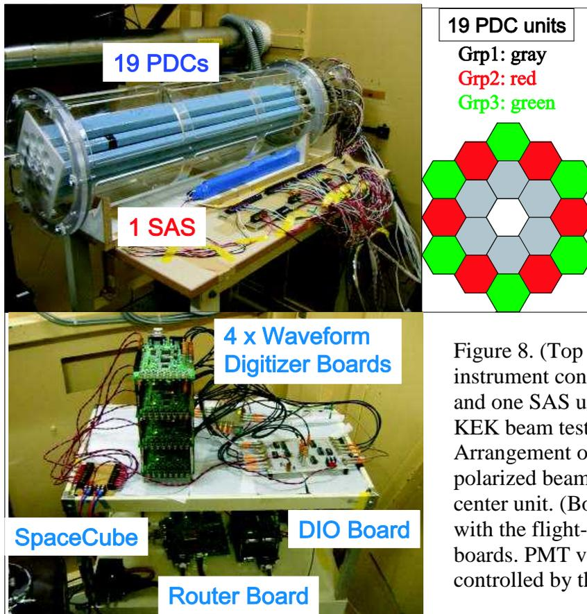
Figure 8. (Top left) Prototype instrument consisting of 19 PDCs and one SAS unit, used in the KEK beam test. (Top right) Arrangement of the 19 PDCs. A polarized beam is irradiated at the center unit. (Bottom) DAQ Setup with the flight-version SpaceWire boards. PMT voltages are also controlled by the digitizer boards.
