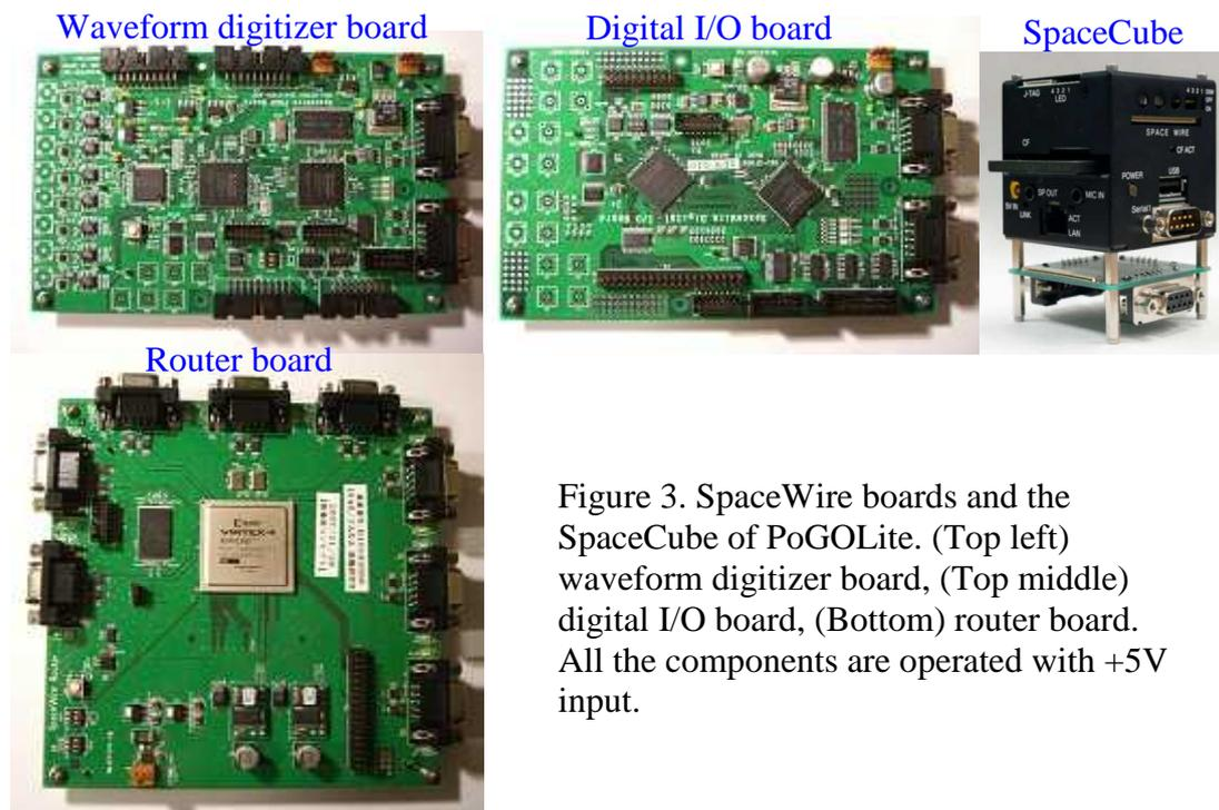
Figure 3. SpaceWire boards and the SpaceCube of PoGOLite. (Top left) waveform digitizer board, (Top middle) digital I/O board, (Bottom) router board. All the components are operated with +5V input.
