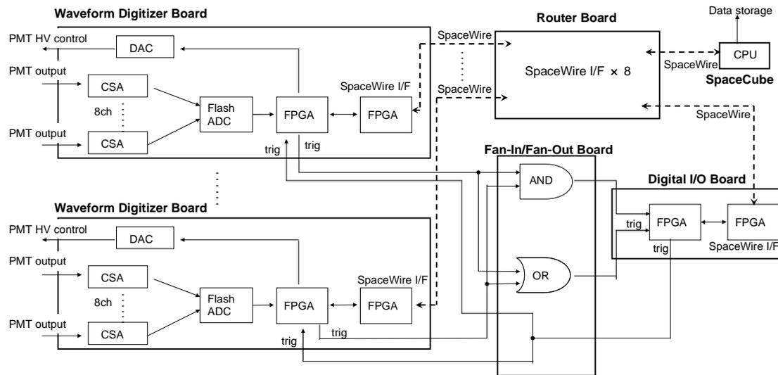
Figure 4. Block diagram of the PoGOLite DAQ system. All waveform digitizer boards and digital I/O boards are controlled and read by the SpaceCube through the router board. The reference voltage to operate each PMT (around +5V) is set by accessing the digitizer board through the SpaceWire connection.
