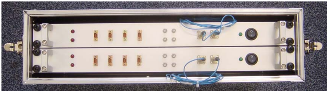
Figure 3: First prototype implementation of one SpaceFibre link and two SpaceWire – SpaceFibre Routers
