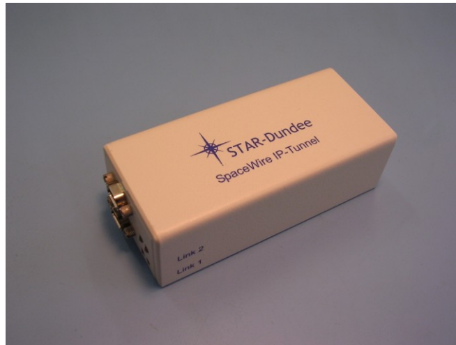
Figure 3: The SpaceWire IP-Tunnel hardware
